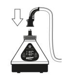
6. Put Tube on Filling Chamber.
